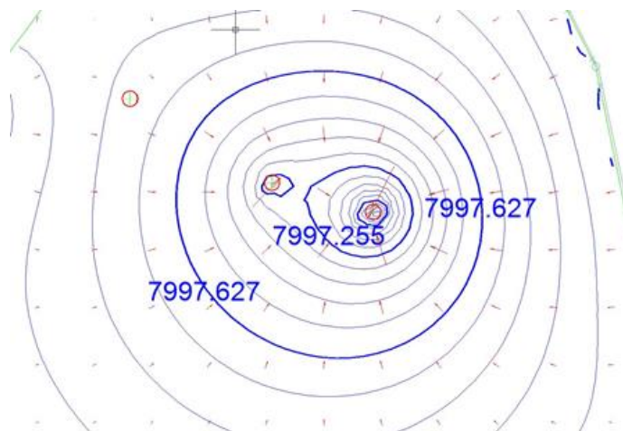
Figure 8: Results from pumping model (close-up)
